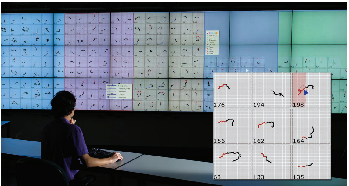
Figure 3. A visualization of ant trajectories on the Cyber-Commons in a 2D layout with stereoscopic depth cues. Trajectories were grouped into bins and collectively analyzed. The inset illustrates the coordinated brushing feature used to formulate and perform quick visual queries.
