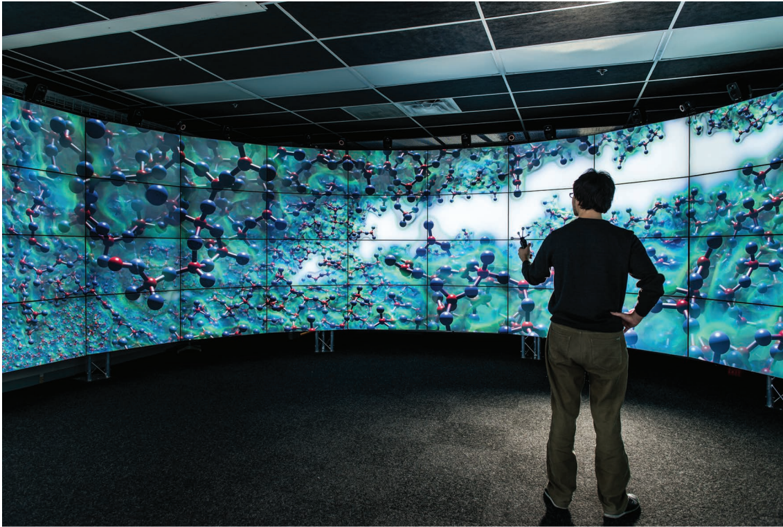
Figure 6. A real-time immersive visualization of a molecular-dynamics simulation of a glass fissure, comprising approximately five million atoms. CAVE2's high resolution allows such massive nanoscale structures to be resolved in stereoscopic 3D.
