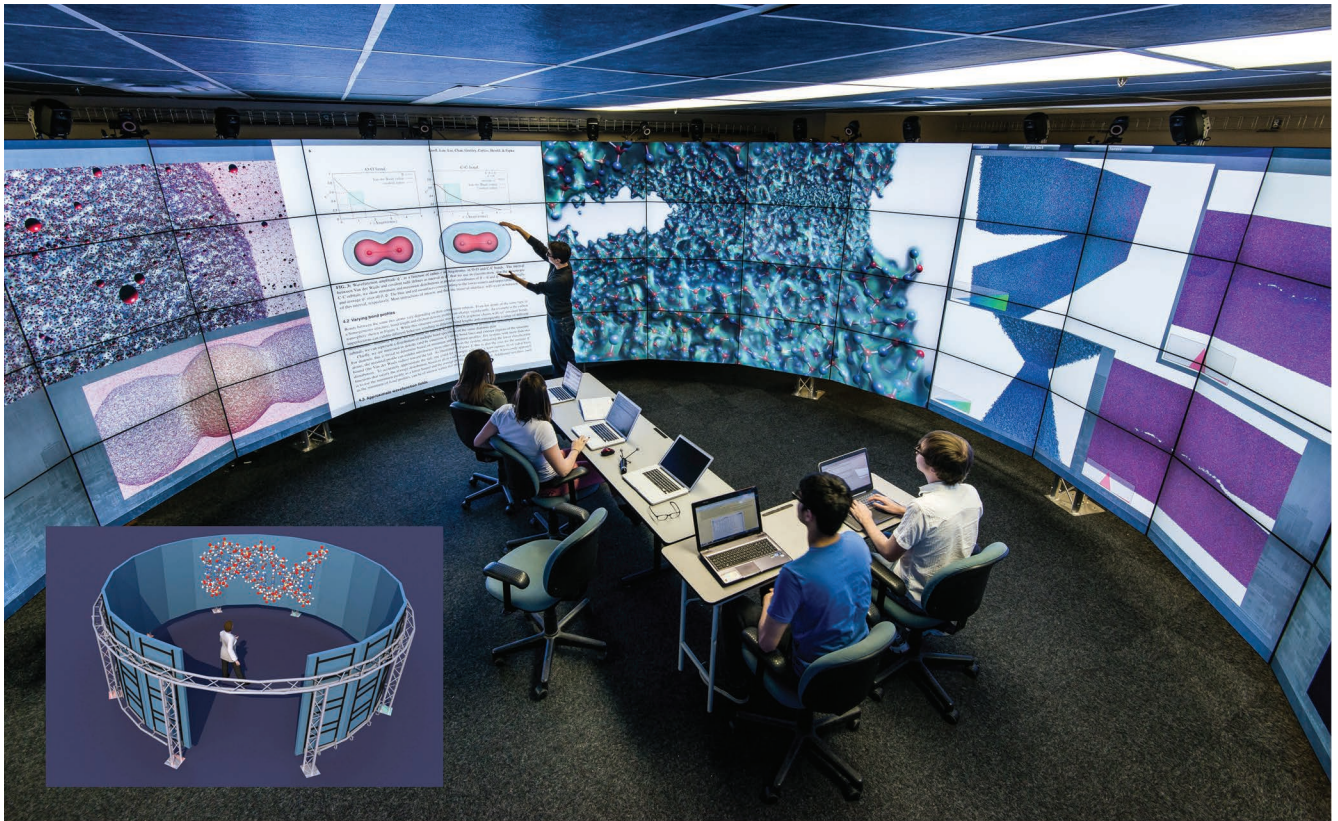
Figure 1. Students having an immersive meeting in CAVE2. The space can comfortably accommodate from five to seven individuals with chairs and tables. CAVE2 can be used to effectively juxtapose 2D, 3D, and abstract data, as well as text documents. It features a 320-degree panoramic view at 20/20 visual acuity. With a total of 72 thin-bezel, stereoscopic LCD panels, it has 10 times the resolution of the original CAVE at half the cost.
