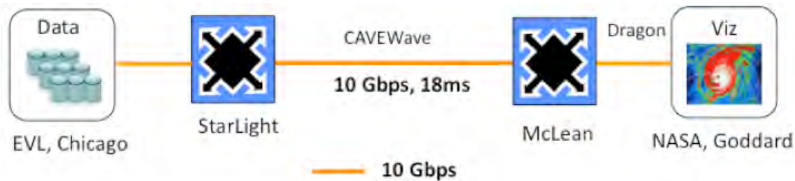
Figure 6: Wide-area 10Gbps testbed to evaluate the performance of accessing data using LambdaRAM to visualize MERRA data. StarLight 4 is a 1 and 10 Gbps network connection point for both national and international research traffic.
